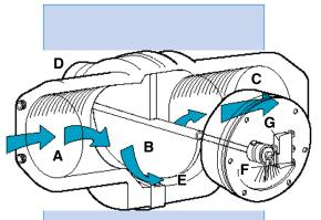
Fluid enters at A, passes around the semi-circular vane B. exits at outlet C. The vane resists the flow because of the spring D. The further the vane is pushed the larger the passageway E becomes. This minimizes pressure drop. The vane shaft turns to operate the pointer F and remote signal devices such as the switch G.
