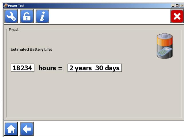
Power tool is a software which allows to evaluate the converter battery life.
