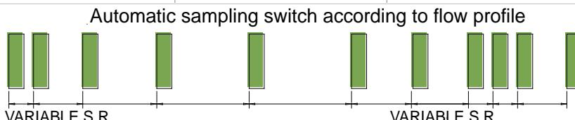
An internal algorithm allows the unit to automatically detect flow rate variations in the process. This capability determines the automatic setting of the sampling frequency. No variations means lower sampling frequency, with less power consumption; high variations means higher frequency to better follows the changes in the process.
