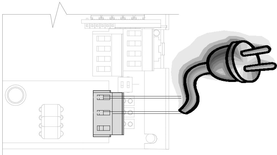
Auto detection of the power source: when main power supply is ON, batteries are excluded and the system always works at the maximum sampling rate (continuous sampling)
